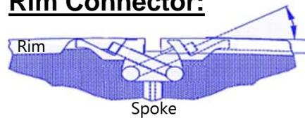
TR Series wheels feature a patented rim and spoke design which allows for each section of the wheel to be tensioned independently. This simplifies field assembly and provides a flatter, rounder and stronger wheel.
