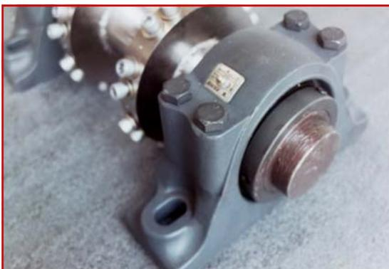
**The hub and bearing assembly support the wheel in the casing.**
